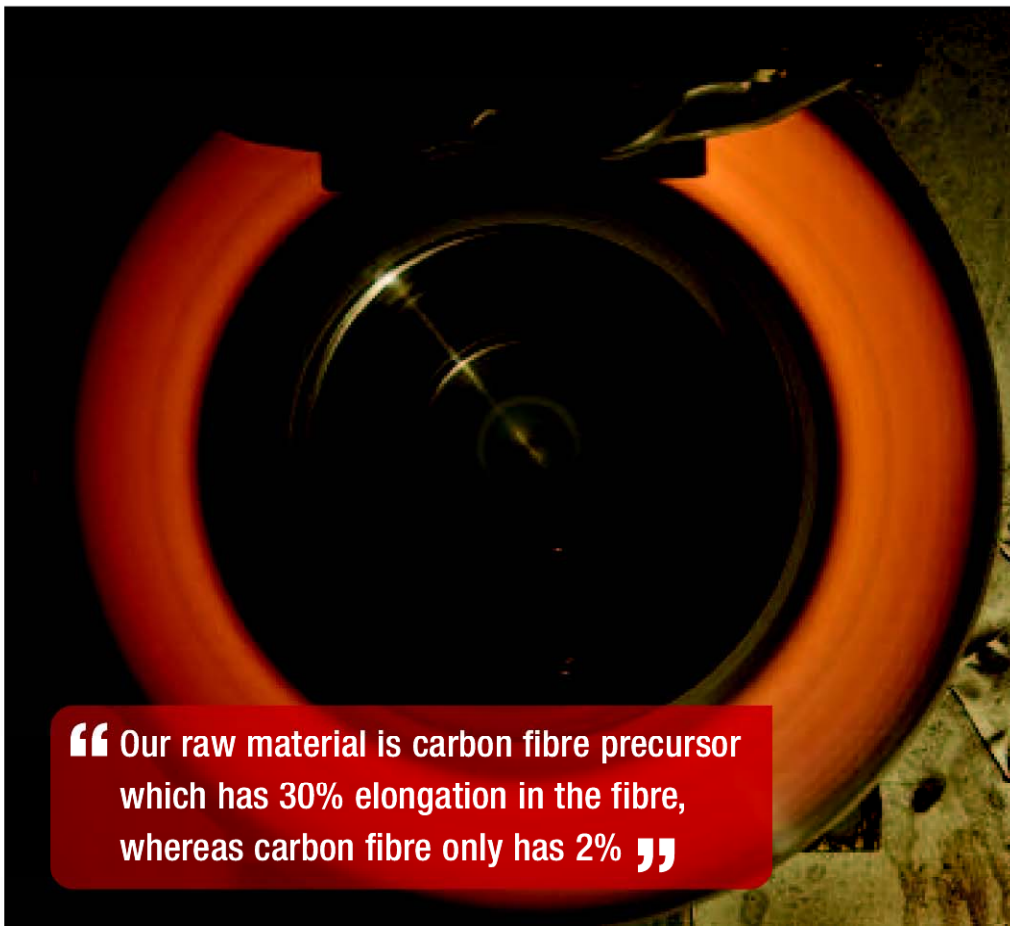
LEFT Surface Transforms SystemST brakes perform to the highest levels, having been developed for over seven years in Formula One, the Indy Racing League and on aircraft. The rotors are ultra lightweight (some 70% lighter than cast iron) and have incredible stopping power. The company believes they offer the best performance, integrity and wear advantages on the market
