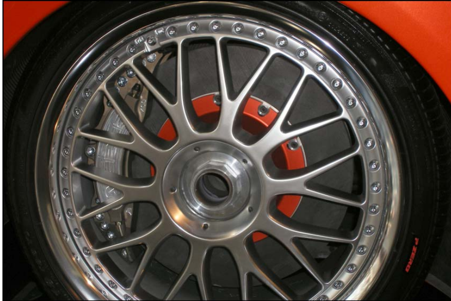
Brake detail of the Weber, showing SystemST ceramic disc
